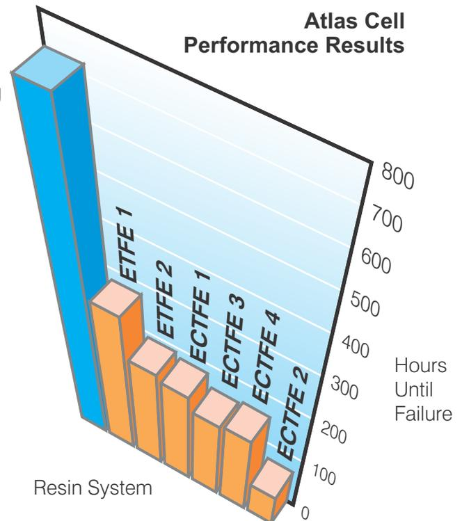
The atlas cell test is an industry standard test per IAW ASTM C 868-85 Standard Test Method for Chemical Resistance of Protective Linings and their adhesion to steel substrates under attack of various solutions at elevated temperatures.
