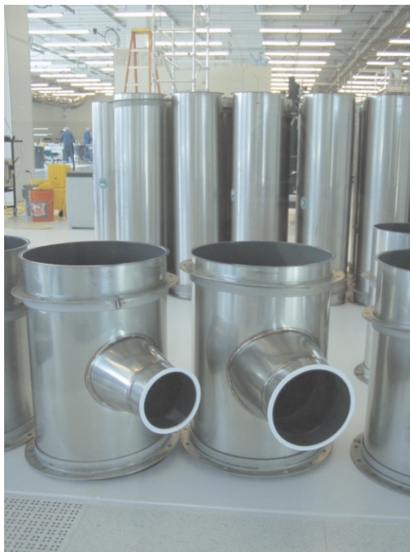
Coated stainless steel exhaust duct staged for installation at a NY State University research center. ( Photo credit V. Rocca, Fab-Tech, Inc. )
